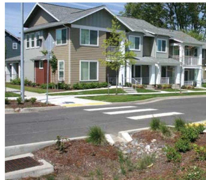
◀ Swales help capture stormwater onsite.
